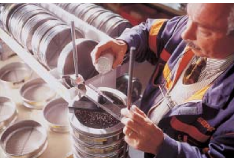
Measurement of the grain size distribution in a sample of beads
