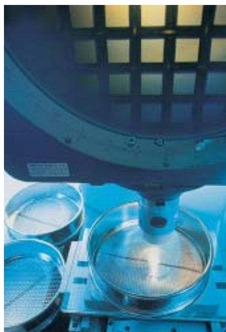
Dimensional inspection of screens used by Quality Control
